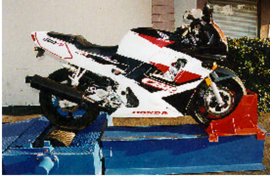
low profile chassis - 1 man loading no need to sink dyno in floor.
