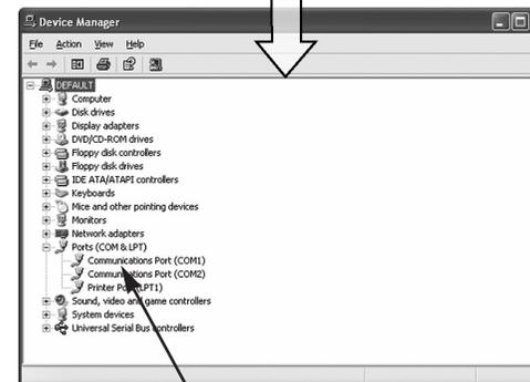
Unable to communicate when the "x" mark is appeared on the communication port (COM1). Also unable to communicate if the COM port is differ from tool setting.
