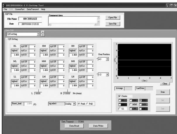
The voltage line of checked trigger will be displayed (Only HH is checked to display the line in the above example).
