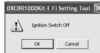
Turn on the engine switch and press "OK" or "Enter" within 2 seconds.
