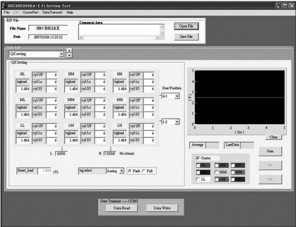
The cyl UP (Upper injector), cyl Lo (Lower injector) and ignition cut-off cycle are set in the condition in the table below.
