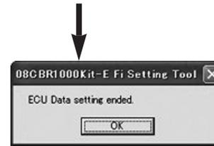
If the communication is correctly completed, the following window will appear. Turn the engine stop switch OFF.
