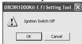
Turn the engine stop switch OFF, click "OK." The following window will appear.
