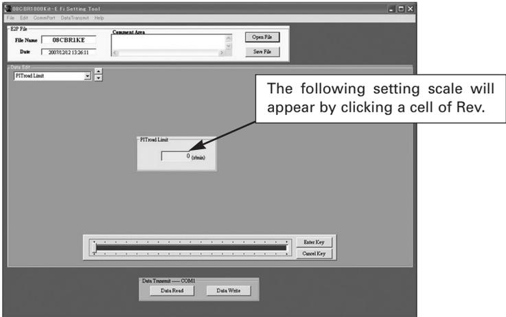
Set the ignition cut engine speed as follows:
