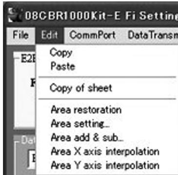
Interpolates cell block data in the specified area.
