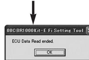
If communication is correctly completed, the following window will appear. Turn the engine stop switch OFF.
