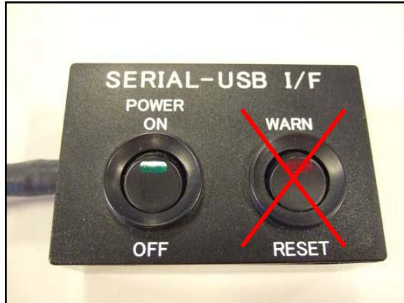
**IMPORTANT:** It is highly recommended that data be **WRITTEN TO** a new ECU before it is ever read. The ECU does not log any data and there is no readable base setting from the factory, so there is nothing to read until a setting is sent.
